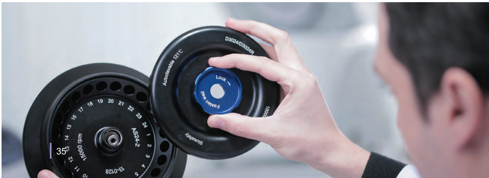
Seals within the aluminum alloy rotor
